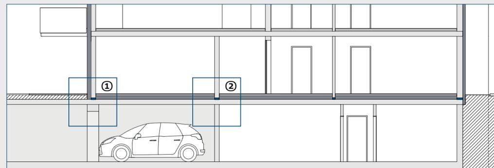
Optimized with Scconnex, insulation completely laid on-slab thickness 130 mm and exposed concrete ceiling.
