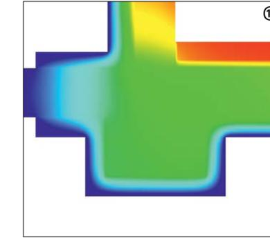
Variant A: Ceiling insulation without Scconnex®
