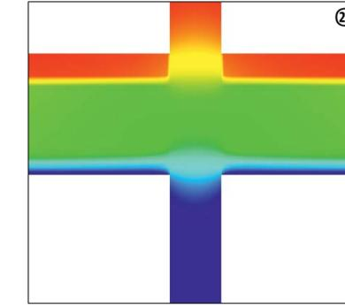
Variant A: Ceiling insulation without Scconnex®
