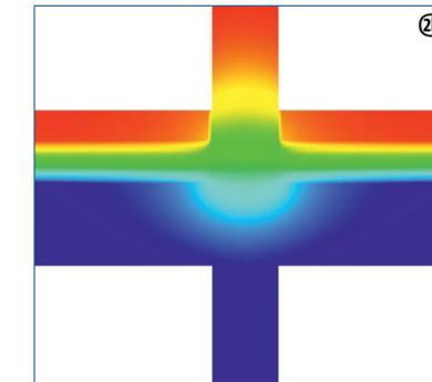
Variant B: No ceiling or flanking insulation
