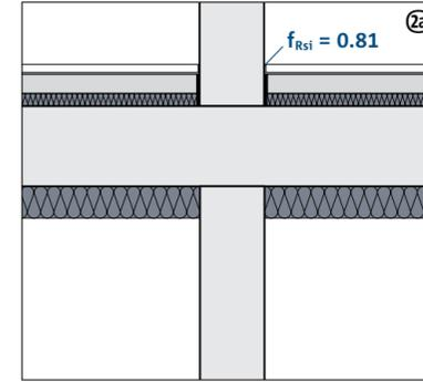
Variant A: Ceiling insulation without Scconnex®
