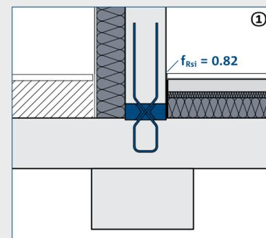
Beam and ceiling exposed concrete finish
