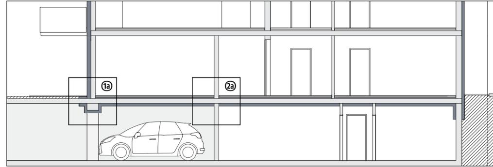
Variant A: Insulation thickness 100 mm below the slab and sound insulation 40 mm above the slab
