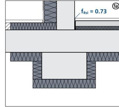
Variant A: Ceiling insulation without Scconnex®
