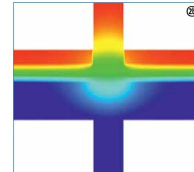
Variant B: No ceiling or flanking insulation
