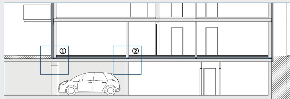
Optimised with Sconnex®, insulation completely laid on-slab thickness 130 mm and exposed concrete ceiling.
