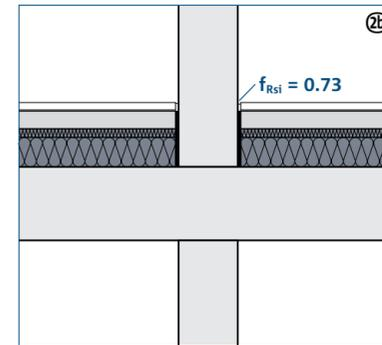
Variant B: No ceiling or flanking insulation
