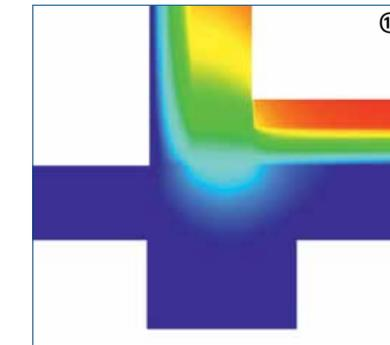
Variant B: No ceiling insulation to the beam
