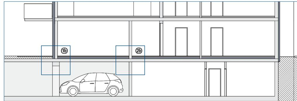
Variant B: Insulation thickness 130 mm above the slab
