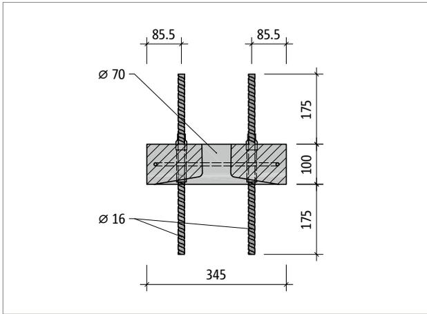
Fig. 155: Schöck Sconnex® type P-B350: Product section Part C
