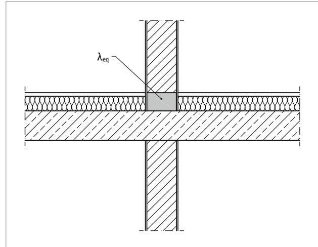
Fig. 55: Representation of a sectional drawing with simplified substitute insulating element
