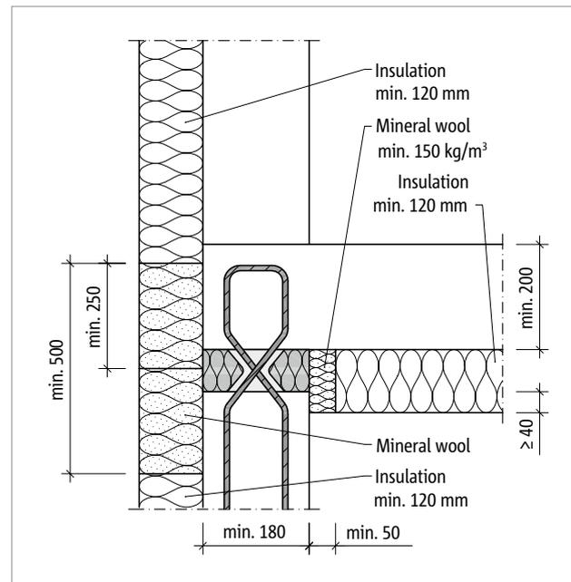
Fig. 104: Schöck Sconnex® type W: For combustible ETICS with fire bar (exterior) and fire protection strips made of mineral wool (interior)
