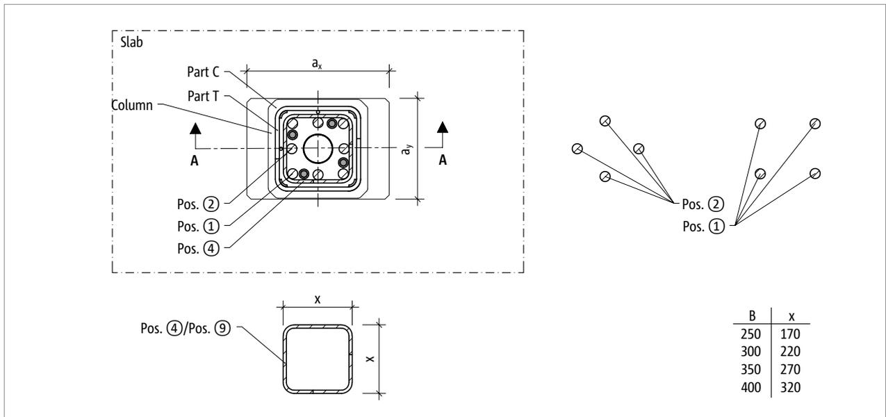
Fig. 174: Schöck Sconnex® type P: On-site reinforcement in column cross-section
