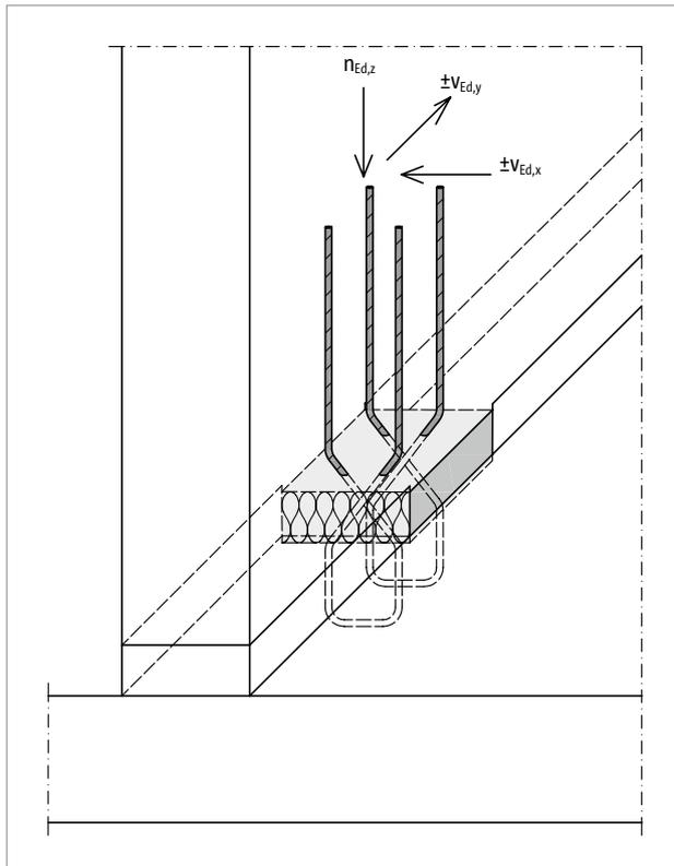
Fig. 115: Schöck Sconnex® type W-N-VH: Static system
