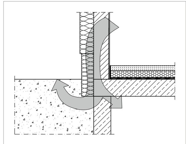
Fig. 51: Structural layout with uninsulated footing
