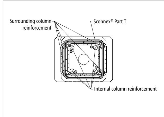
Fig. 168: Schöck Sconnex® type P: Reinforcement layout in Area 2 - column cross-section
