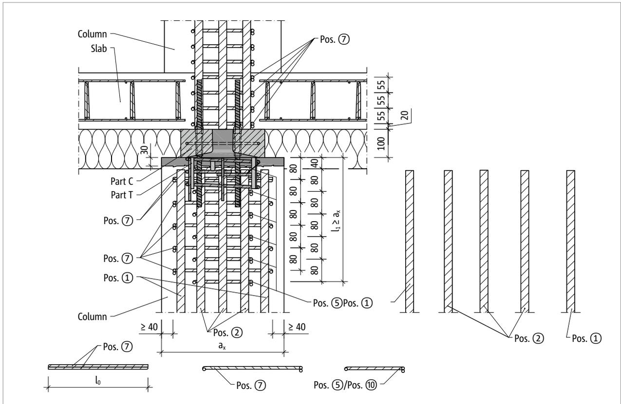
Fig. 177: Schöck Sconnex® type P: On-site reinforcement in column cross-section A-A
