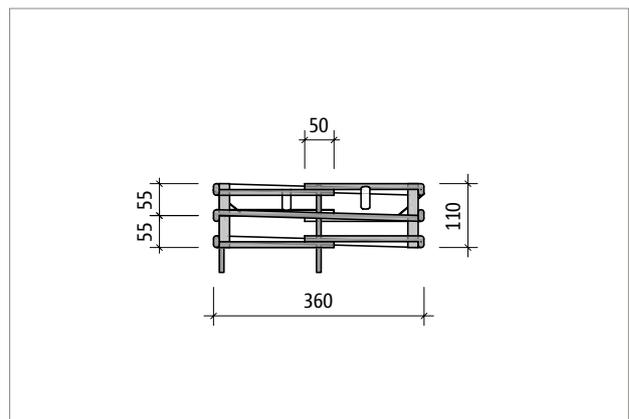
Fig. 164: Schöck Sconnex® type P-B400: Side view Part T; welded stirrup and bending form segments made of stainless steel
