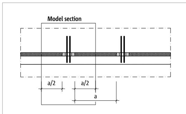
Fig. 43: Representation of a possible model section for a three-dimensional modelling of a wall connection detail with point-sited Schöck Sconnex® type W and insulation in between
