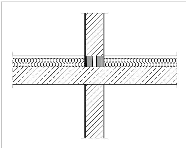
Fig. 38: Representation of a sectional drawing with detailed Schöck Sconnex® model
