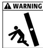
**Danger of tilting due to articulated connection at the bottom of the wall!** In all construction conditions secure walls on Sconnex® type W against tilting!
