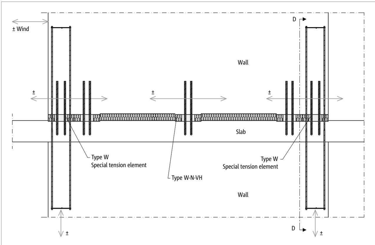
Fig. 66: Schöck Scconnex® type W: Combined product variants for the connection of a horizontal, loaded, stabilized wall
