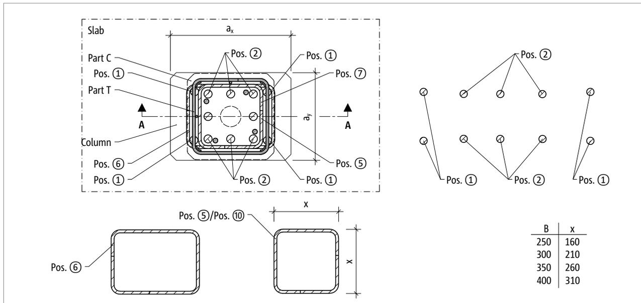
Fig. 176: Schöck Scconnex® type P: On-site reinforcement in column cross-section
