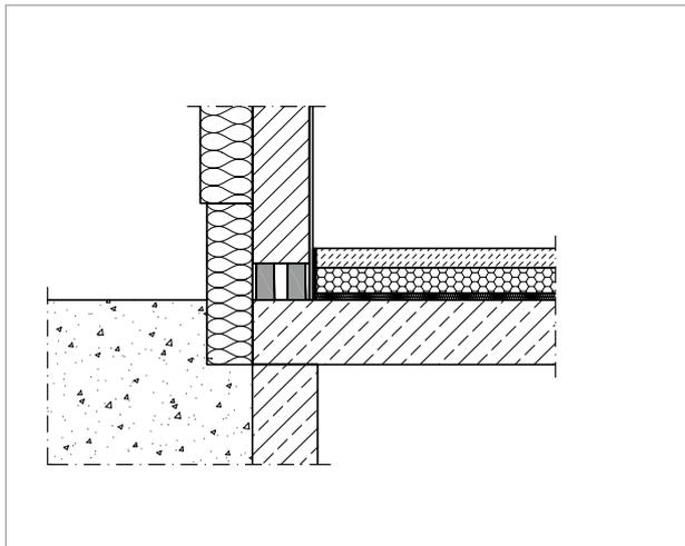
Fig. 49: Efficient thermal insulation using Schöck Sconnex® type M
