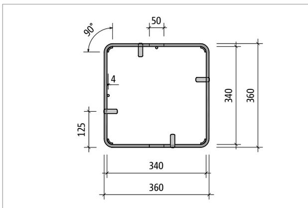
Fig. 163: Schöck Sconnex® type P-B400: Part T; welded stirrup and bending mould segment made of stainless steel
