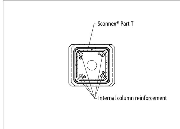
Fig. 166: Schöck Sconnex® type P: Reinforcement layout in Area 1 - column cross-section
