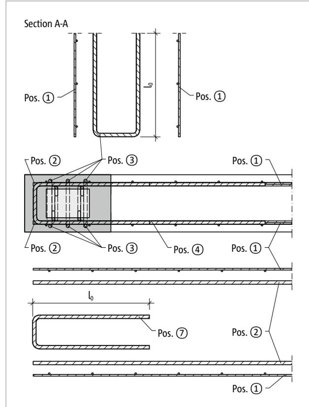
Fig. 110: Schöck Scconnex® type W-N-VH: Variant A – on-site reinforcement with Pos. 4 for connection to end of wall
