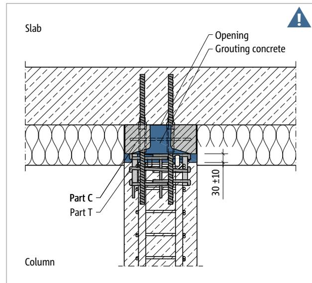
Fig. 180: Schöck Sconnex® type P: Installation section; connection column – floor using form fit to the column concrete using PAGEL® grouting V1/50
