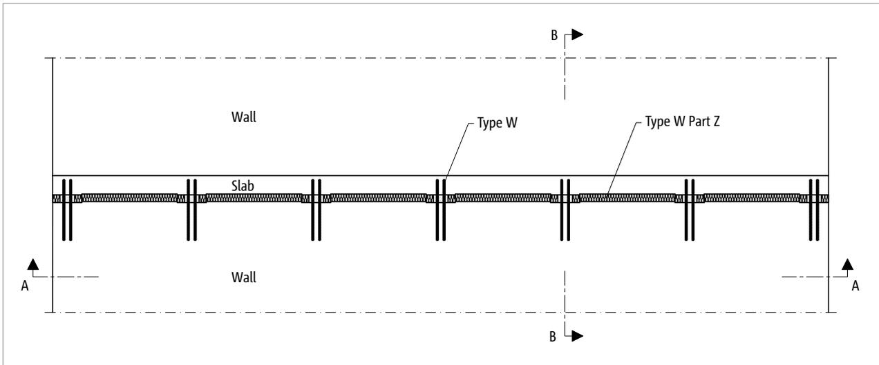
Fig. 56: Schöck Sconnex® type W: Connection between wall and slab above – installation at the top of the wall
