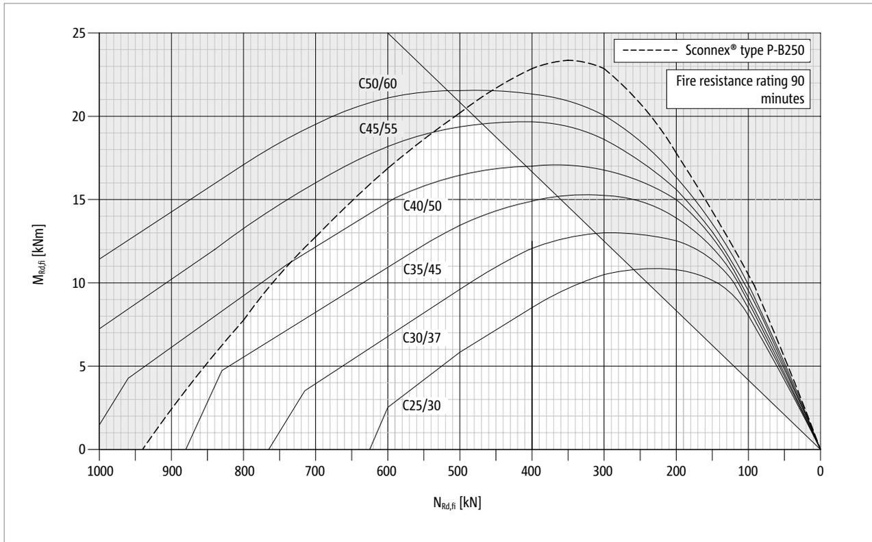
Fig. 129: Schöck Sconnex® type P-B250: Interaction diagram for the dimensioning for the case of fire, fire resistance class R 90
