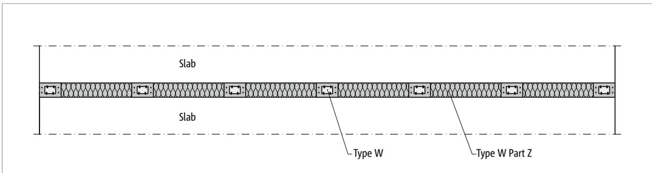
Fig. 58: Schöck Sconnex® type W: Section A-A
