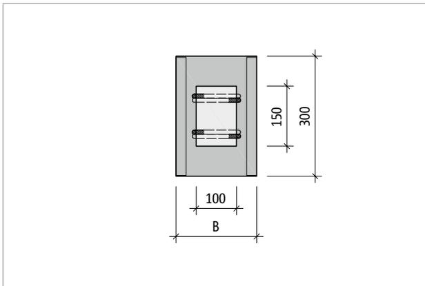
Fig. 82: Schöck Sconnex® type W-N-VH: Product plan view; pressure bearing area 150 mm x 100 mm
