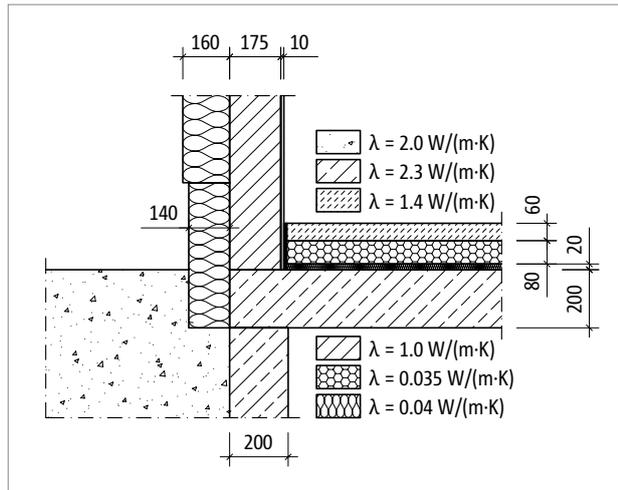
Fig. 50: Structural layout with uninsulated footing
