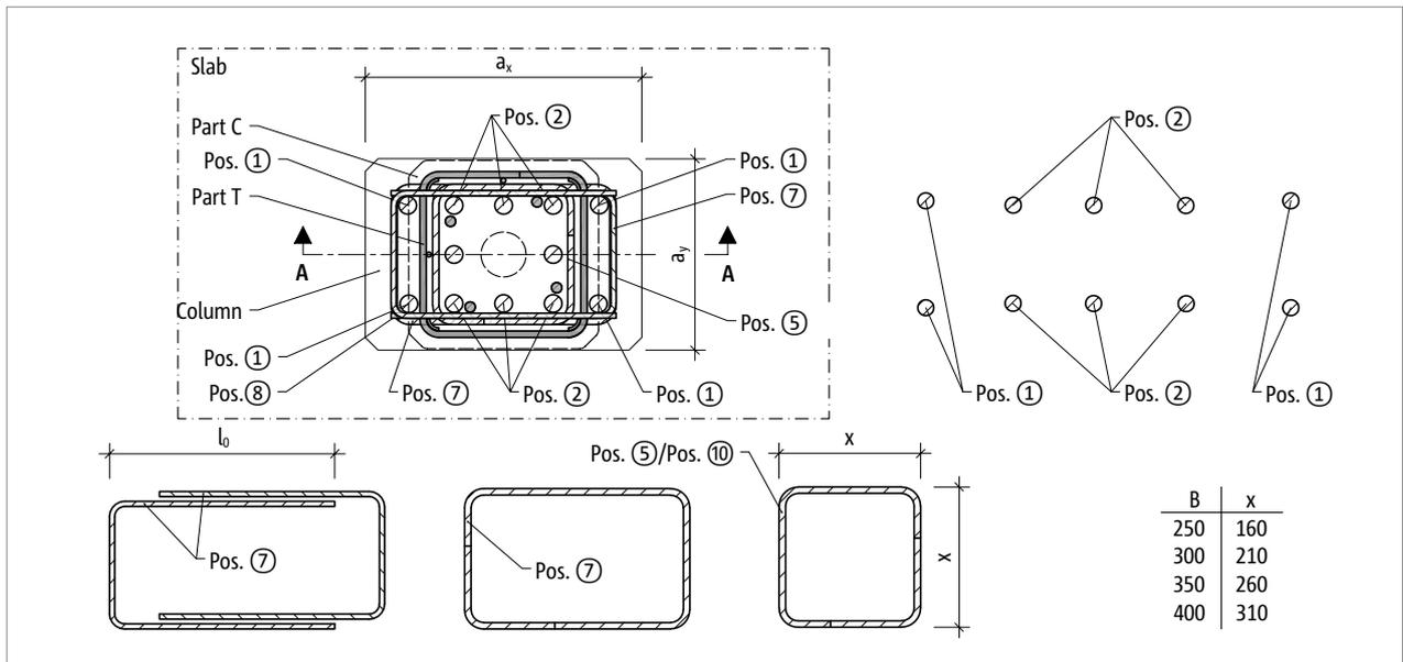
Fig. 178: Schöck Sconnex® type P: On-site reinforcement in column cross-section
