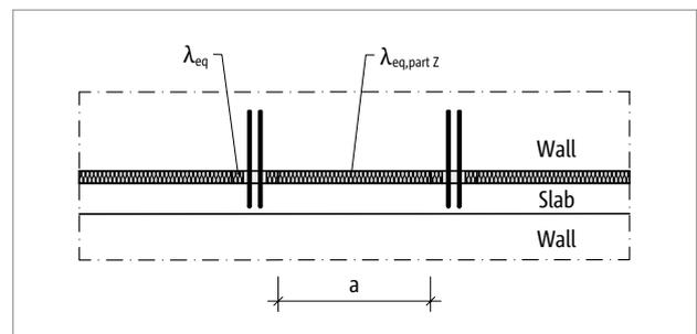
Fig. 44: Representation of two sectional axes for the determination of  $\lambda_{eq,mean}$  of a wall connection detail with point-sited Schöck Sconnex® type W and insulation in between
