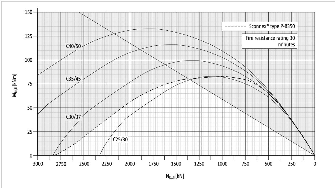
Fig. 137: Schöck Sconnex® type P-B350: Interaction diagram for the dimensioning for the case of fire, fire resistance class R 30
