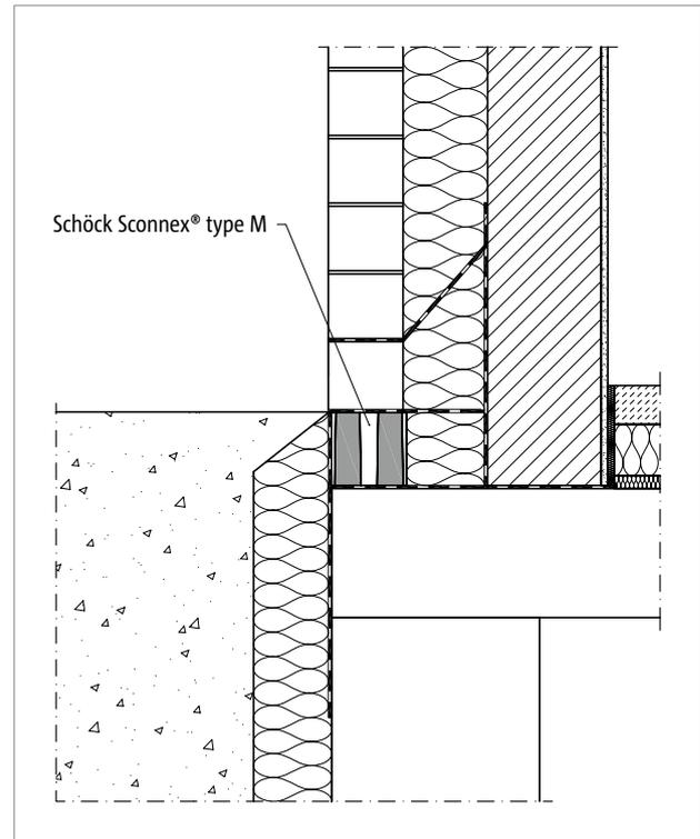
Fig. 186: Schöck Sconnex® type M: Connection with double-leaf masonry
