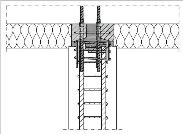
Fig. 165: Schöck Sconnex® type P: Reinforcement layout in Area 1 - longitudinal column section
