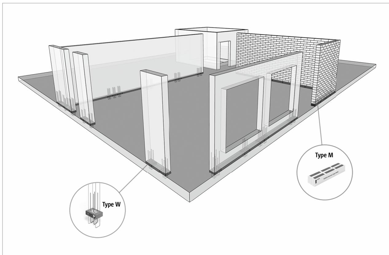
Fig. 2: Above-slab insulation using Schöck Sconnex®
