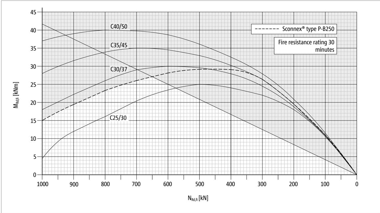
Fig. 131: Schöck Sconnex® type P-B250: Interaction diagram for the dimensioning for the case of fire, fire resistance class R 30
