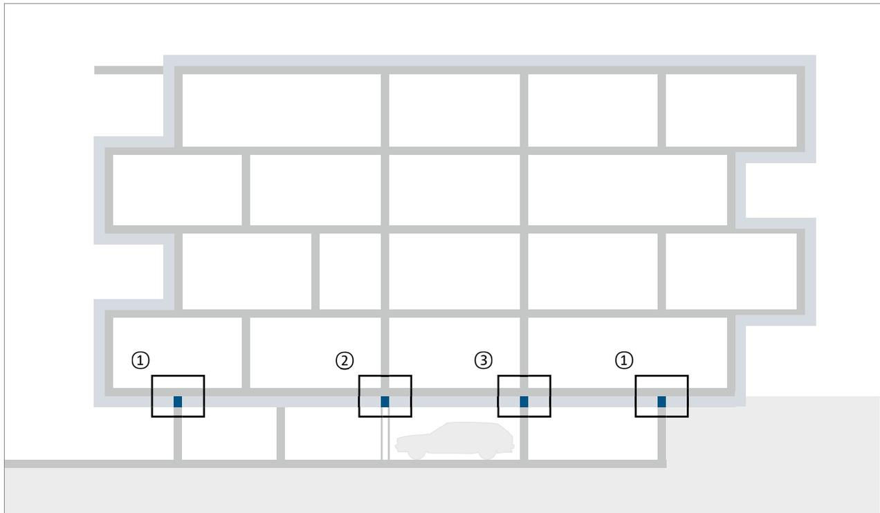
The thermal bridge can be efficiently insulated using the Schöck Sconnex® in the top of walls and columns. The floor located in the thermal zone and the thermal bridges in walls and columns minimized by Schöck Sconnex® leads to an insulation concept that is optimal from a building physics point of view, in which flank insulation is dispensed with and at the same time prevents building damage due to condensation and mould.
