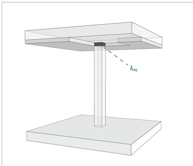
Fig. 47: Connection detail with simplified substitute insulation element
