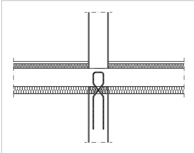
Fig. 41: Representation of a sectional drawing with detailed Schöck Sconnex® model
