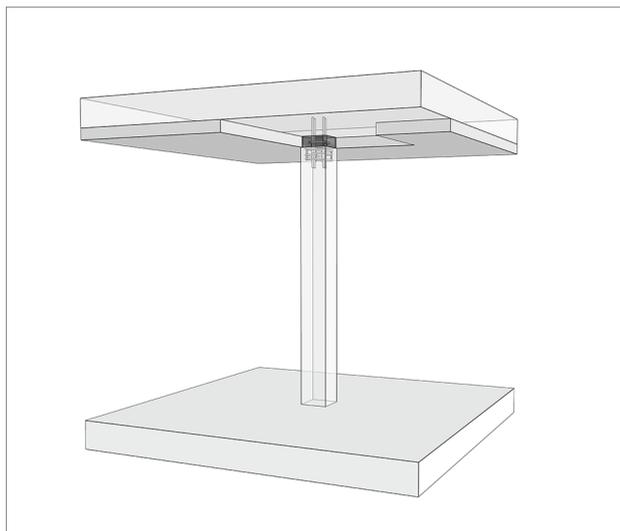
Fig. 46: Connection detail with detailed Schöck Sconnex® model
