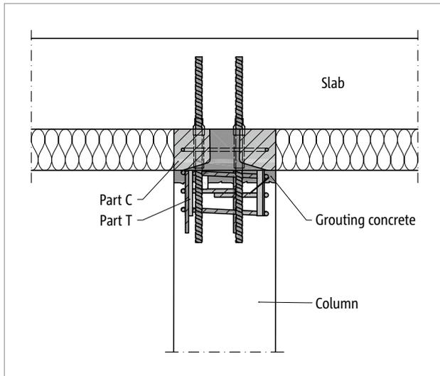
Fig. 121: Schöck Sconnex® type P: Installation section; connection for square column - floor with Part C and Part T
