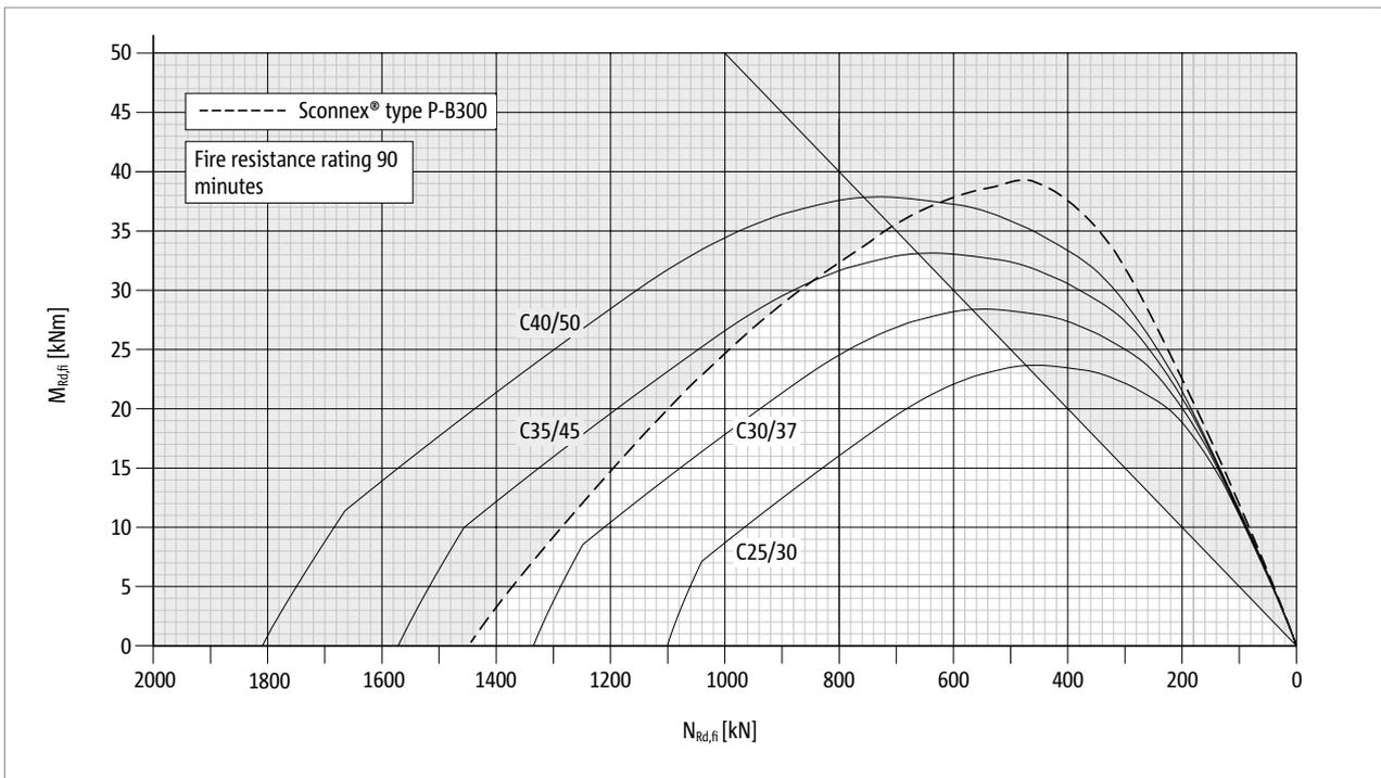
Fig. 132: Schöck Sconnex® type P-B300: Interaction diagram for the dimensioning for the case of fire, fire resistance class R 90
