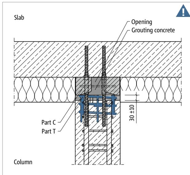
Fig. 179: Schöck Sconnex® type P: Installation section; connection column – floor using integrated Part T for the load-bearing safety in combination with Part C
