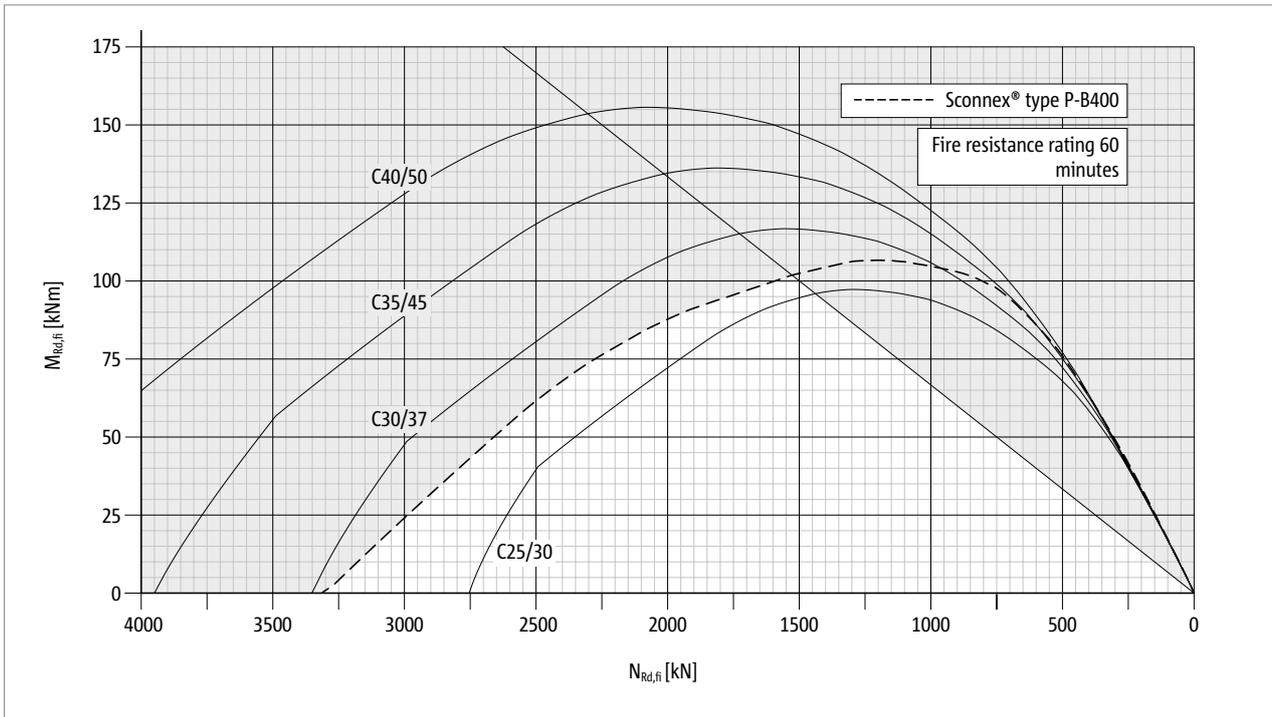
Fig. 139: Schöck Sconnex® type P-B400: Interaction diagram for the dimensioning for the case of fire, fire resistance class R 60
