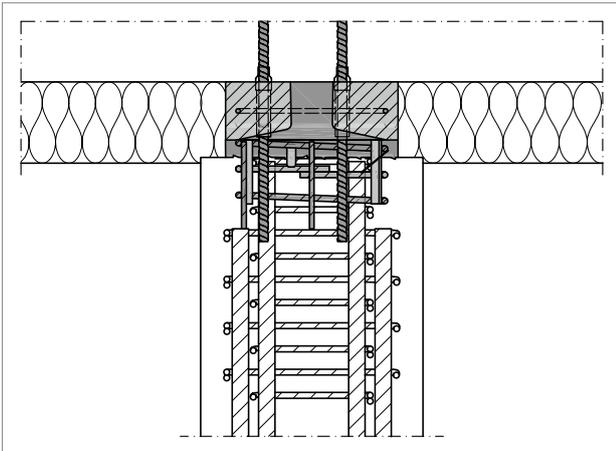
Fig. 167: Schöck Sconnex® type P: Reinforcement layout in Area 2 - longitudinal column section
