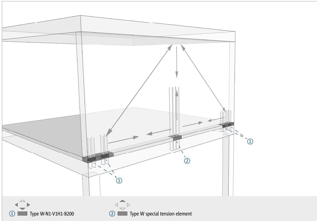
Fig. 77: Wall-type beam separated at the floor
