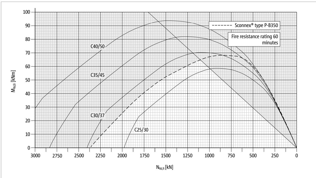
Fig. 136: Schöck Sconnex® type P-B350: Interaction diagram for the dimensioning for the case of fire, fire resistance class R 60
