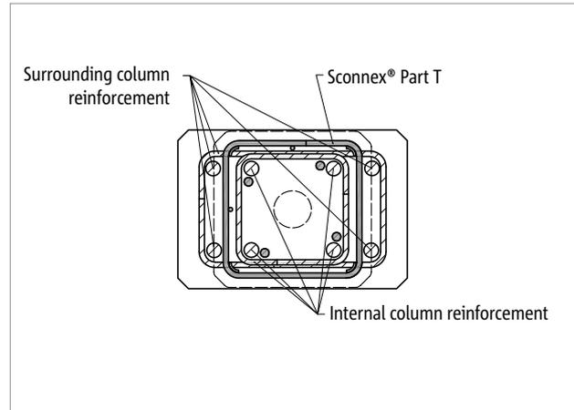
Fig. 170: Schöck Sconnex® type P: Reinforcement layout in Area 3 - column cross-section
