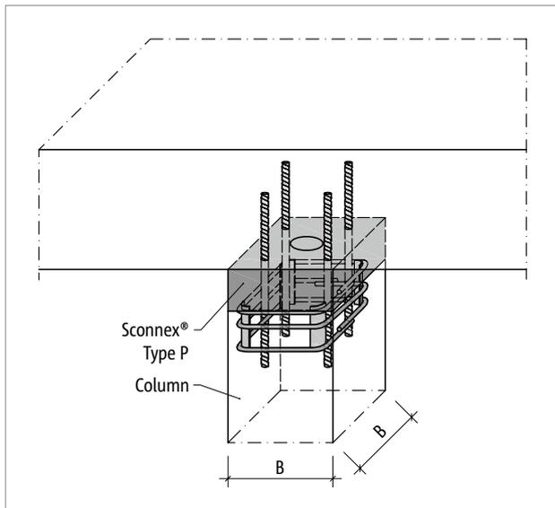
Fig. 123: Schöck Sconnex® type P: Connection for square column
