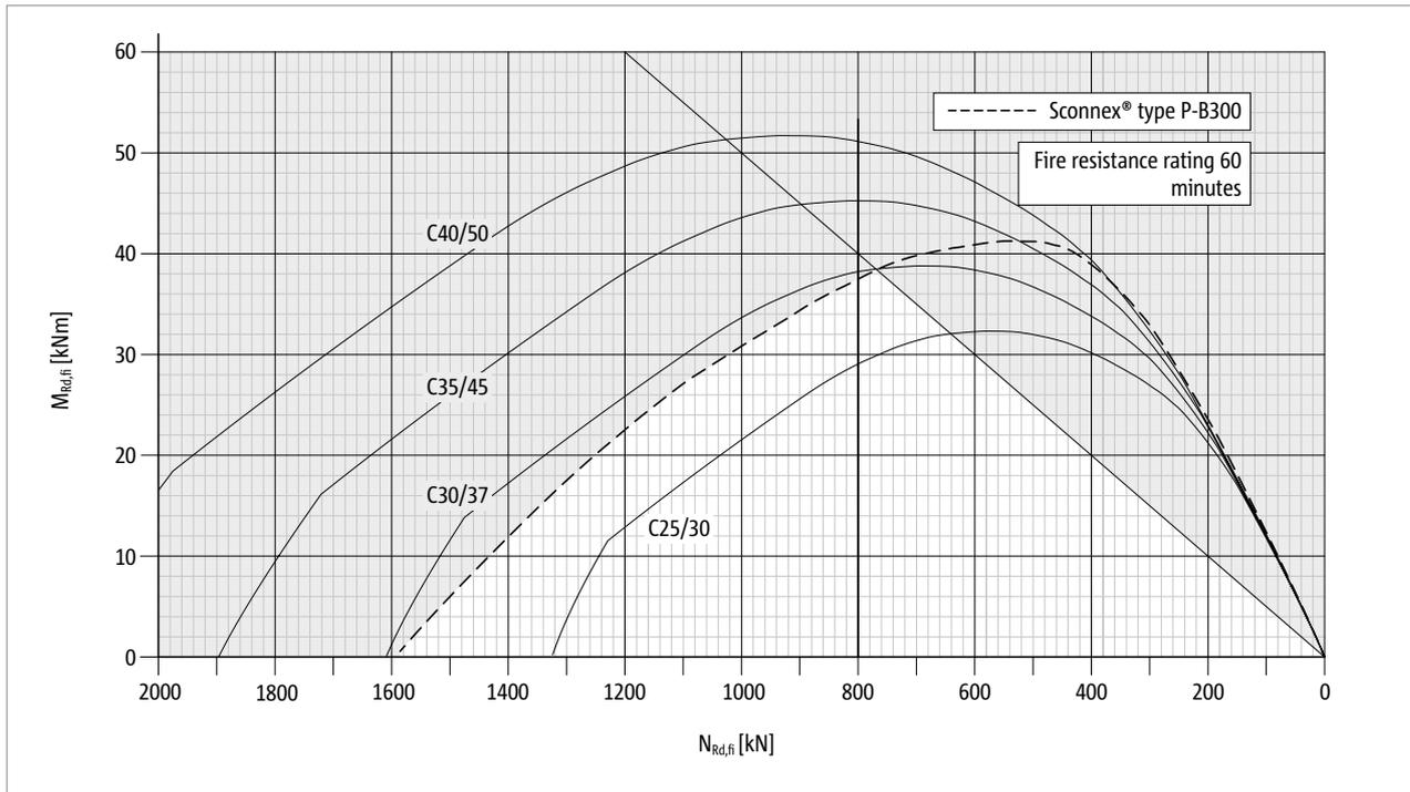
Fig. 133: Schöck Sconnex® type P-B300: Interaction diagram for the dimensioning for the case of fire, fire resistance class R 60
