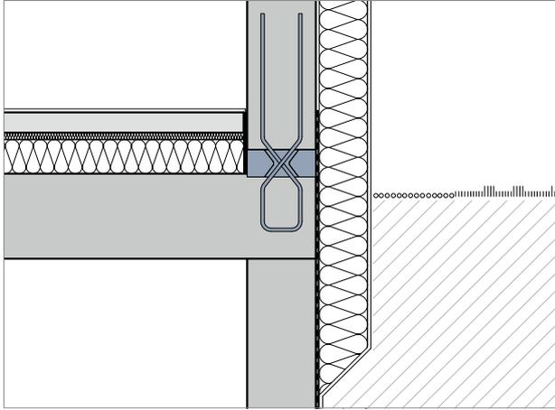
For the exterior wall against the soil, make sure that the joint is adequately protected against moisture penetration by an exterior sealing membrane. In the example presented the element is located in the splash water zone. In order to have a barrier against moisture and fire at the same time, the use of non-combustible, moisture-resistant and insulating materials is recommended in this area.
