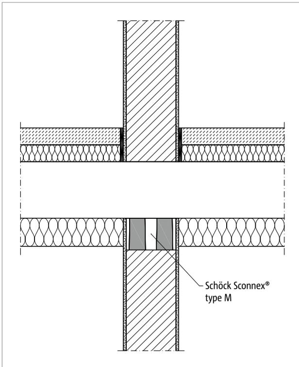
Fig. 189: Schöck Sconnex® type M: Installation condition with interior wall and under-slab installation
