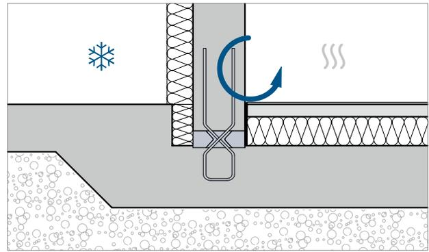
Fig. 9: Pos. ①: Heat flow in underground garage wall with Schöck Sconnex® type W
