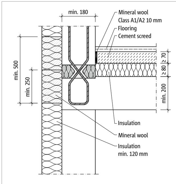
Fig. 98: Schöck Scconnex® type W: For combustibles ETICS with mineral wool fire bar
