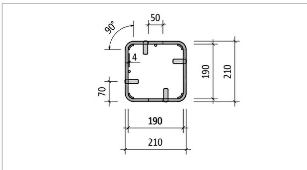
Fig. 145: Schöck Sconnex® type P-B250: Part T; welded stirrup and bending mould segment made of stainless steel
