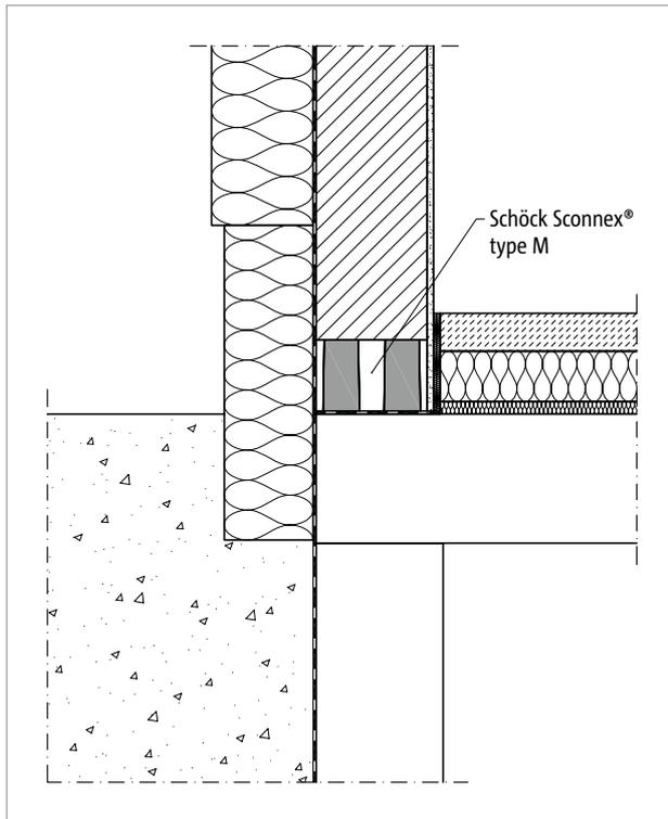
Fig. 185: Schöck Sconnex® type M: Installation condition for external thermal insulation composite system
