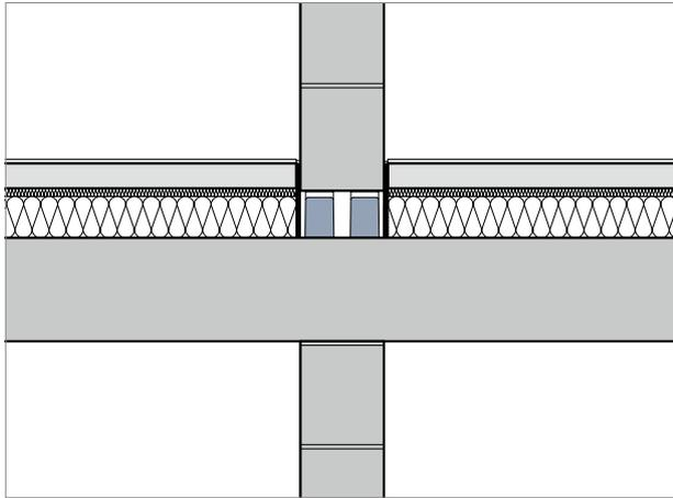
Fig. 25: Schöck Sconnex® type M in masonry with internal walls and above-slab insulation
