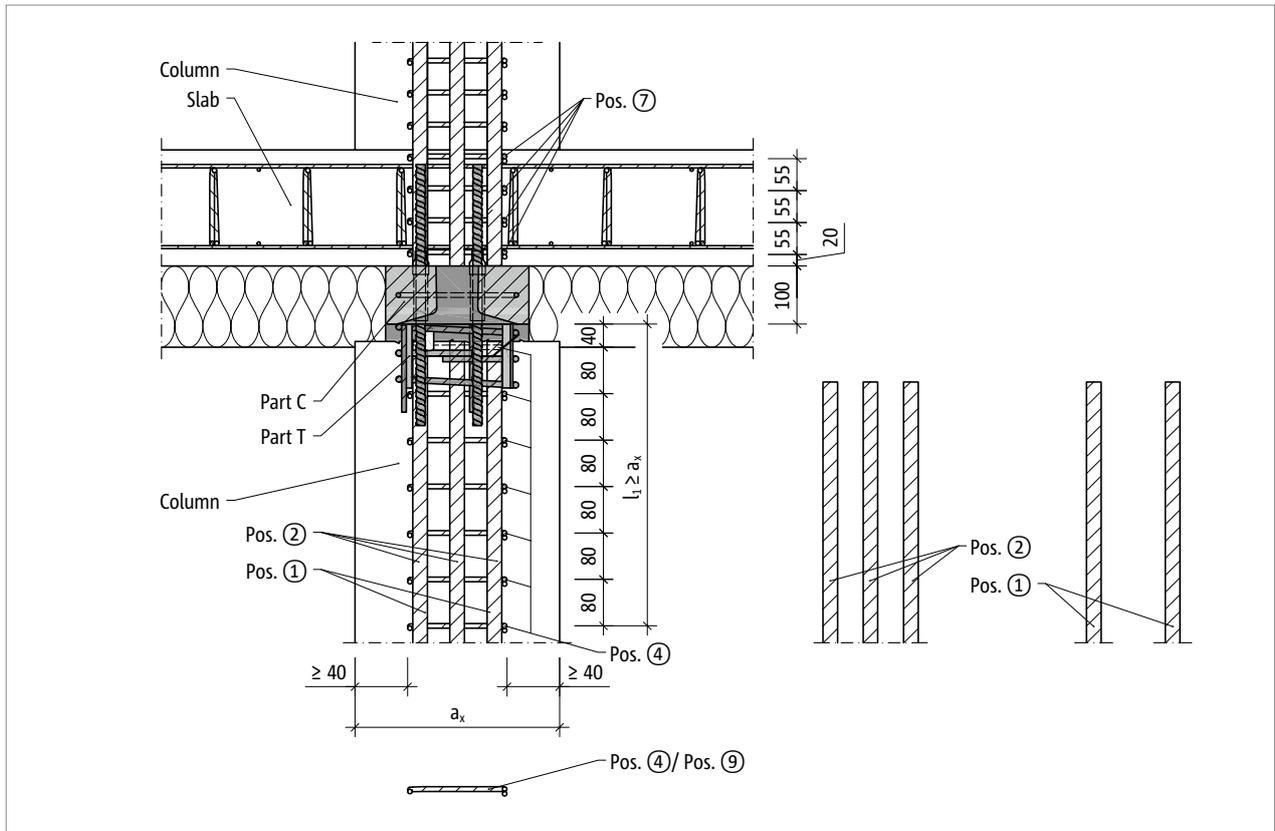
Fig. 173: Schöck Sconnex® type P: On-site reinforcement in column cross-section A-A
