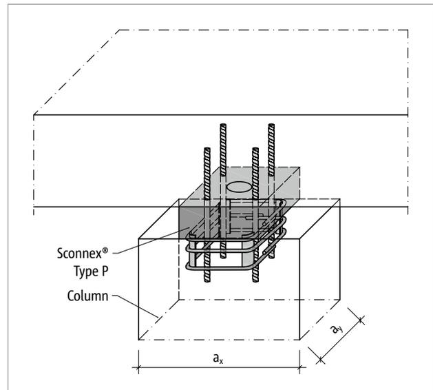
Fig. 124: Schöck Sconnex® type P: Connection for rectangular column; central installation - column dimensions  $a_x$  and  $a_y$ , see page 92
