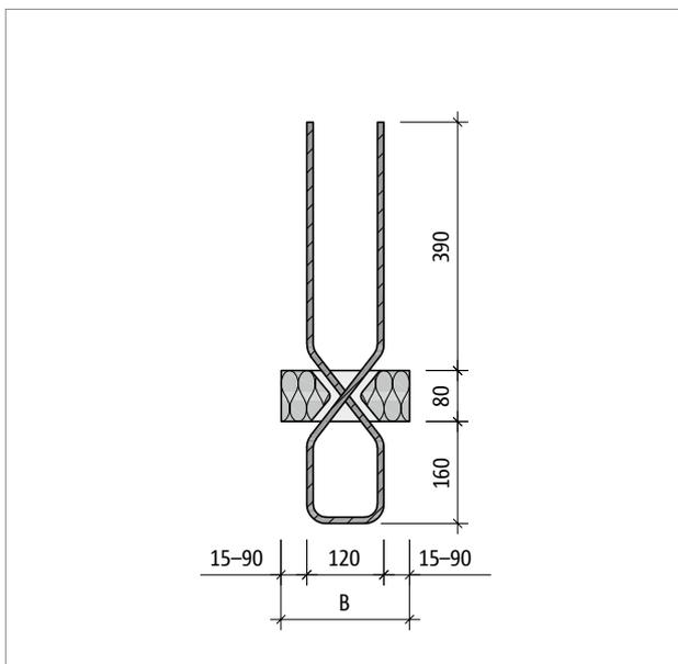
Fig. 89: Schöck Sconnex® type W-N-VH: Product section A-A
