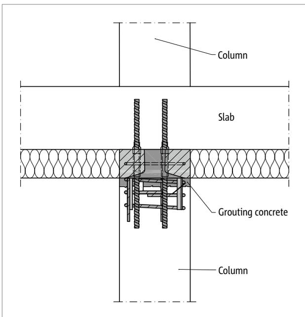
Fig. 119: Schöck Sconnex® type P: Connection of an internal column to the above lying floor
