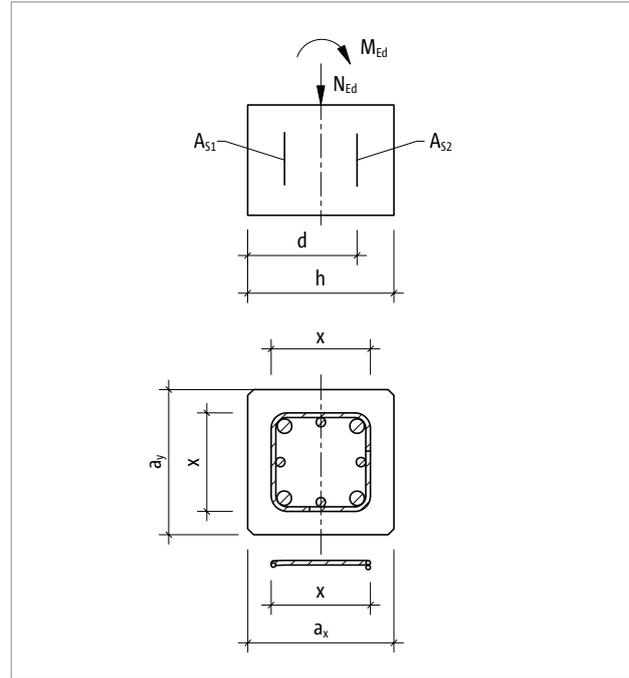
Fig. 127: Schöck Sconnex® type P: Limitation of the external dimension of the stirrups; see warning note ( x - see page 110)
