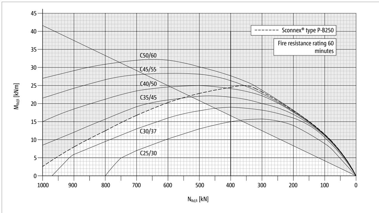
Fig. 130: Schöck Sconnex® type P-B250: Interaction diagram for the dimensioning for the case of fire, fire resistance class R 60
