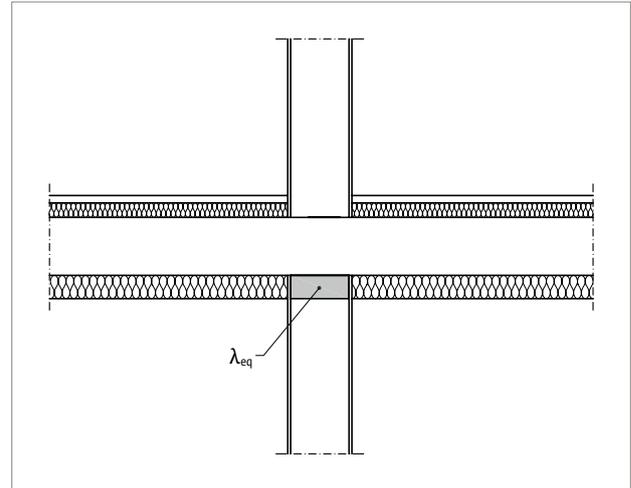
Fig. 42: Representation of a sectional drawing with simplified substitute insulating element
