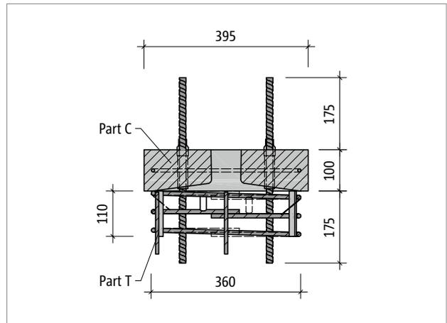
Fig. 162: Schöck Sconnex® type P-B400: Product section Part C and part T
