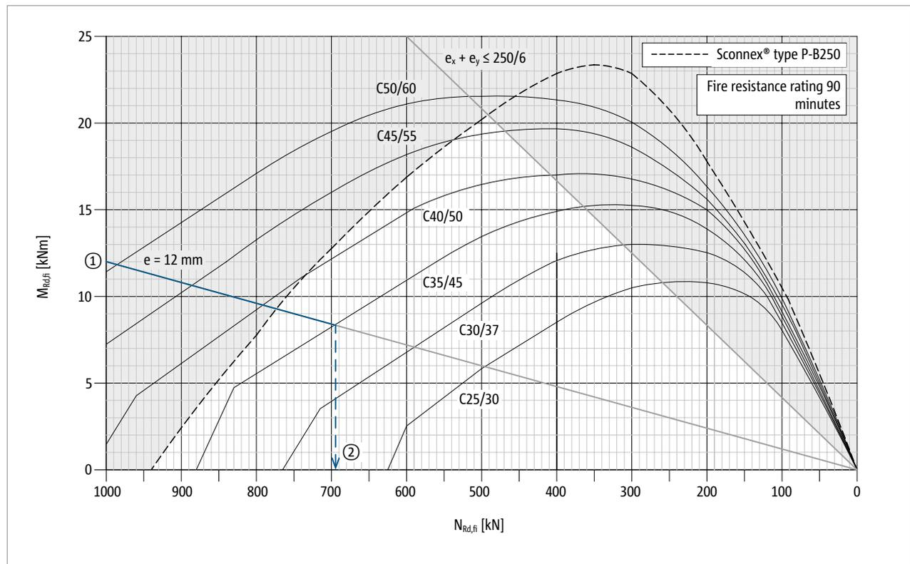
Fig. 184: Schöck Sconnex® type P-B250: Interaction diagram for the dimensioning for the case of fire, fire resistance class R 90
