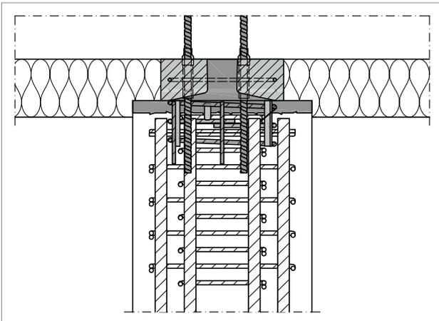
Fig. 169: Schöck Sconnex® type P: Reinforcement layout in Area 3 - longitudinal column section
