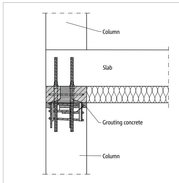
Fig. 120: Schöck Sconnex® type P: Connection of an edge column to the above lying floor
