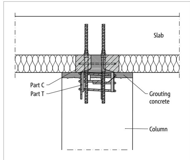
Fig. 122: Schöck Sconnex® type P: Installation section; connection for rectangular column - floor with Part C and Part T
