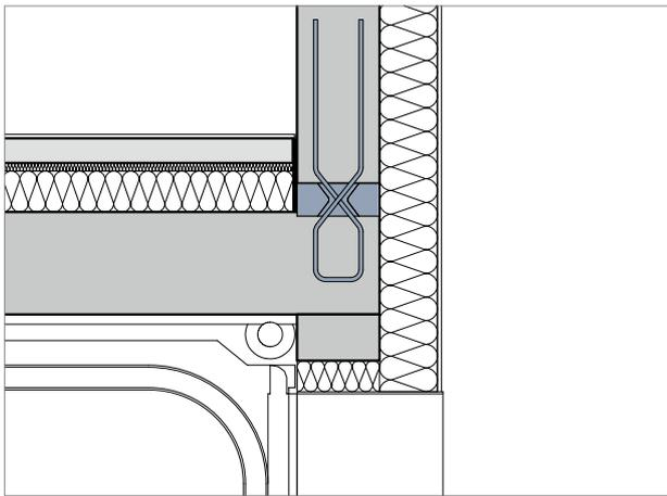
Schöck Sconnex® type W is particularly suitable in areas where the temperature differences between indoor and outdoor air are very large (for example in the area of the underground car park entrance). In order to avoid a thick insulating material surrounding the structure, the main insulation layer can be laid on the inside and through the arrangement of Schöck Sconnex® type W the resultant thermal bridge in the connection detail to the external wall can be solved directly.
