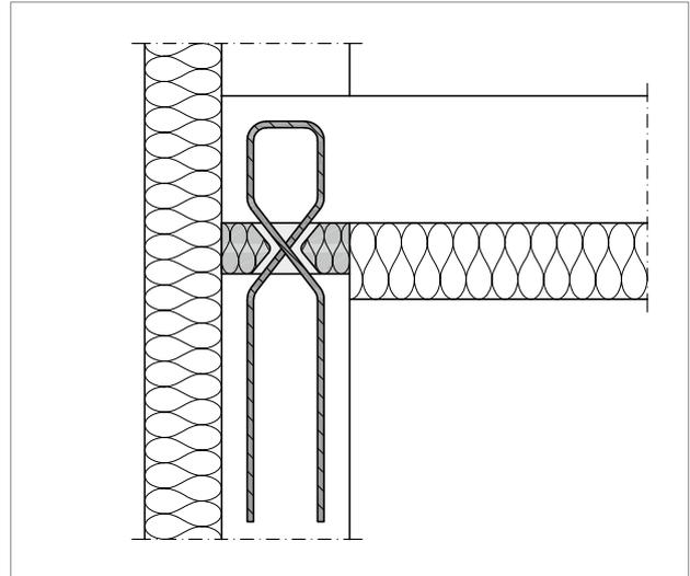
Fig. 60: Schöck Sconnex® type W-N-VH: External wall; below-slab insulation corresponding to Section B-B
