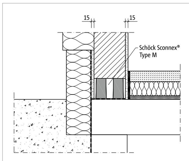
Fig. 192: Schöck Sconnex® type M: REI 30 or REI 90 configuration for technical fire protection integrity
