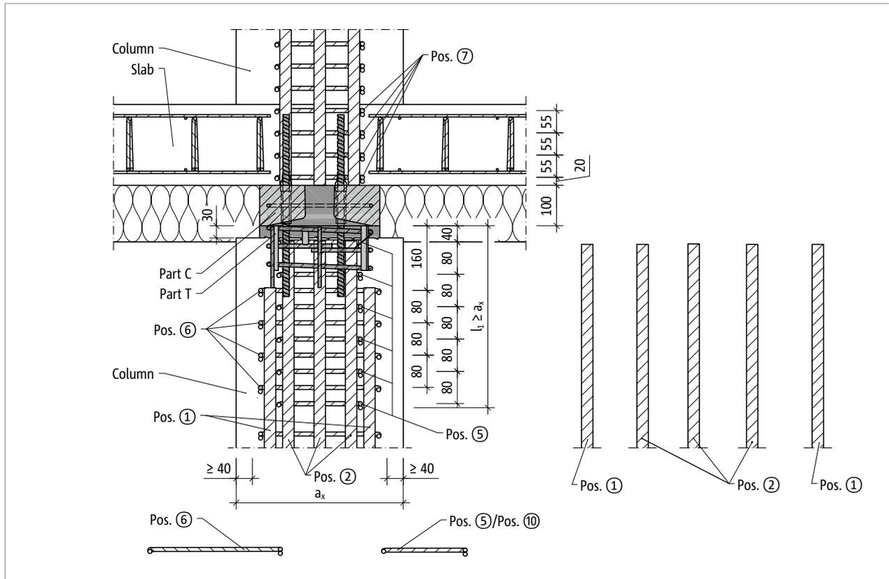
Fig. 175: Schöck Scconnex® type P: On-site reinforcement in column cross-section A-A
