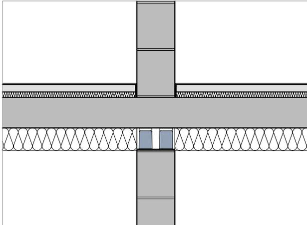
Fig. 48: Schöck Sconnex® type M in masonry with internal walls and under-slab insulation
