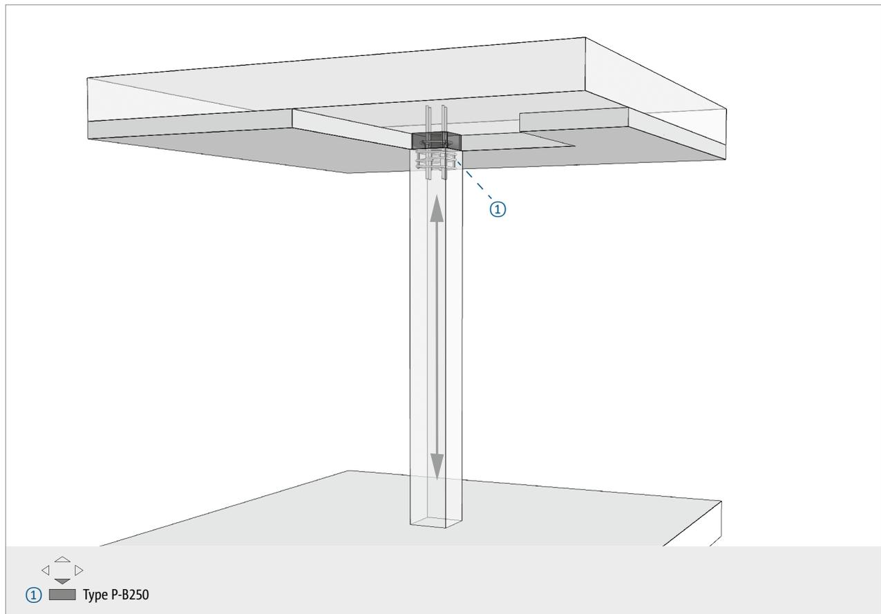
Fig. 125: Column connection with under-slab insulation
