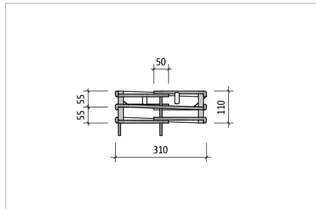
Fig. 158: Schöck Sconnex® type P-B350: Side view Part T; welded stirrup and bending form segments made of stainless steel
