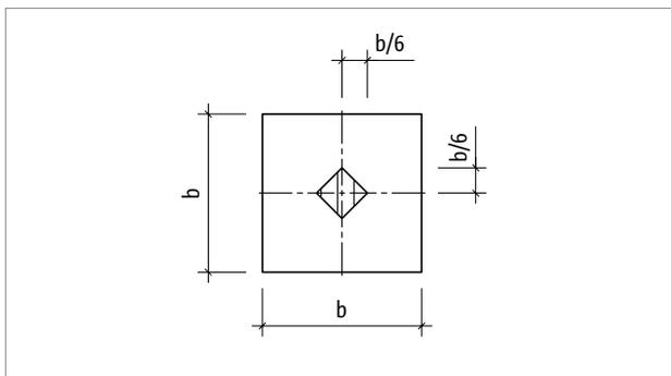
Fig. 128: Schöck Sconnex® type P: Limitation of the eccentricity on the core area of the column cross-section with  $e_x + e_y \leq b/6$ , gapping joint not permitted
