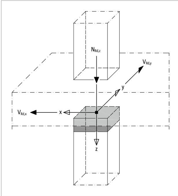
Fig. 126: Schöck Sconnex® type P: Sign convention for the design
