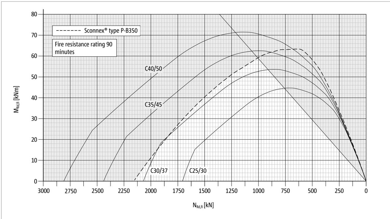
Fig. 135: Schöck Sconnex® type P-B350: Interaction diagram for the dimensioning for the case of fire, fire resistance class R 90
