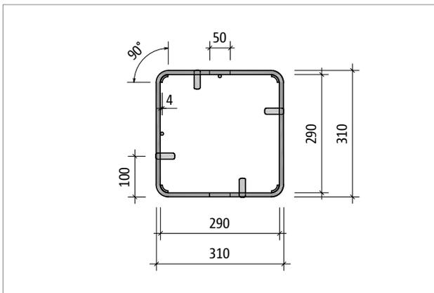
Fig. 157: Schöck Sconnex® type P-B350: Part T; welded stirrup and bending mould segment made of stainless steel
