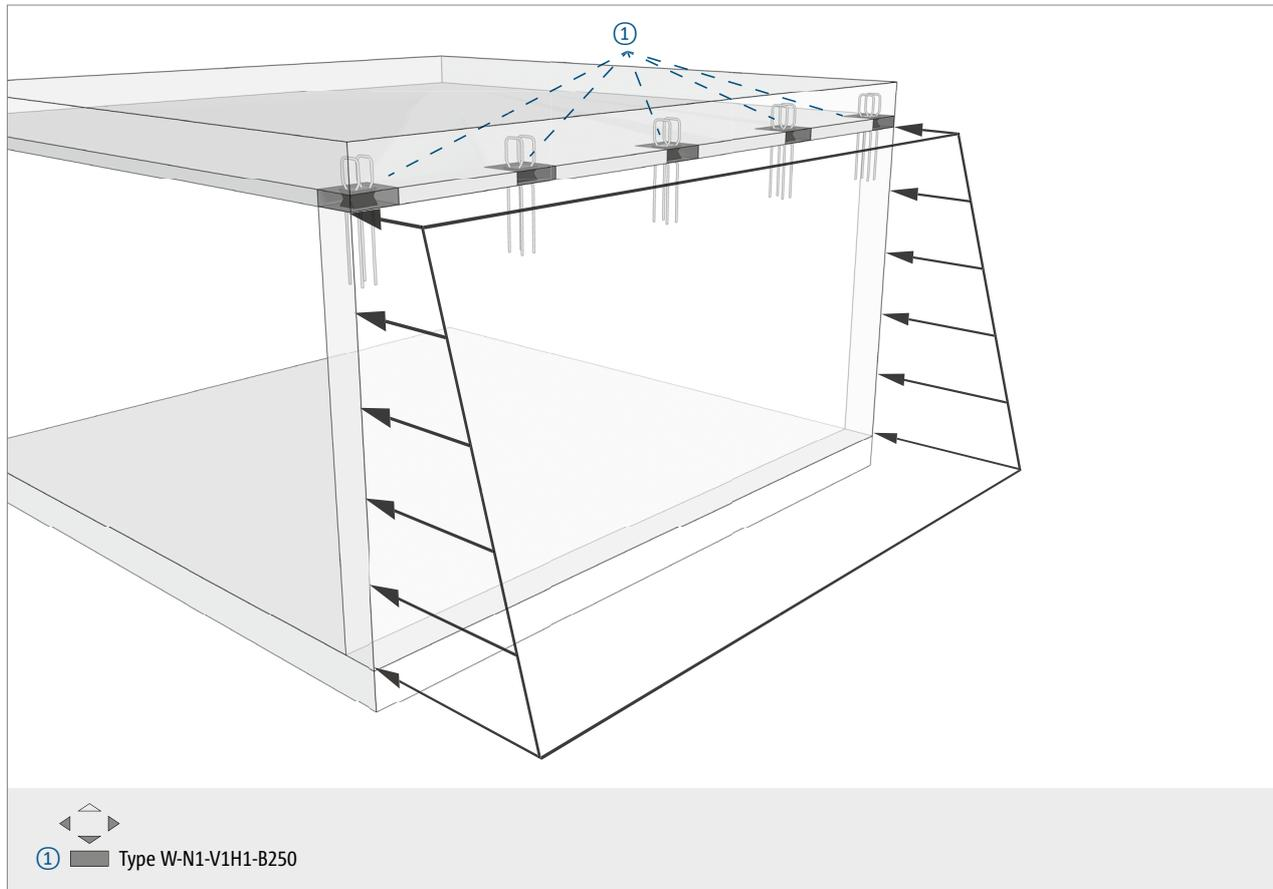
Fig. 74: Earth pressure loaded wall separated below floor
