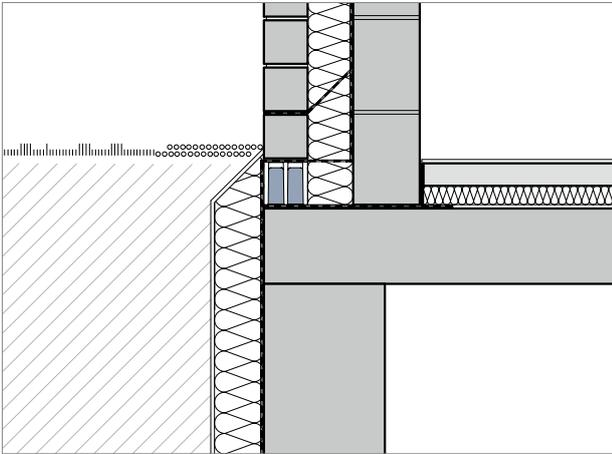
Fig. 31: Schöck Sconnex® type M with double-leaf masonry
