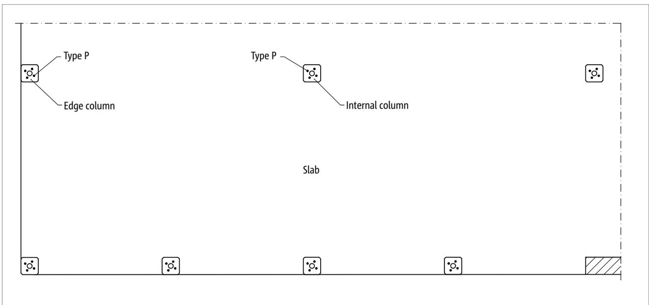
Fig. 118: Schöck Sconnex® type P: Element arrangement in the floor plan
