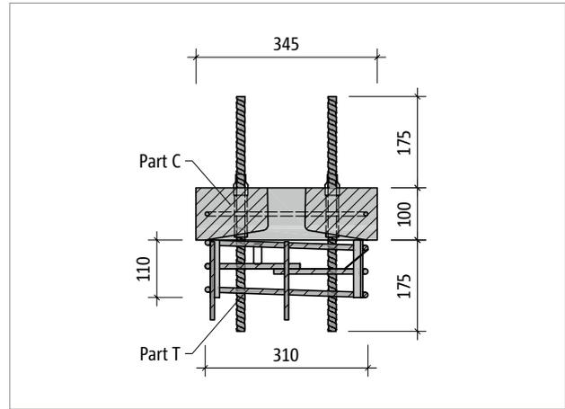
Fig. 156: Schöck Sconnex® type P-B350: Product section Part C and part T
