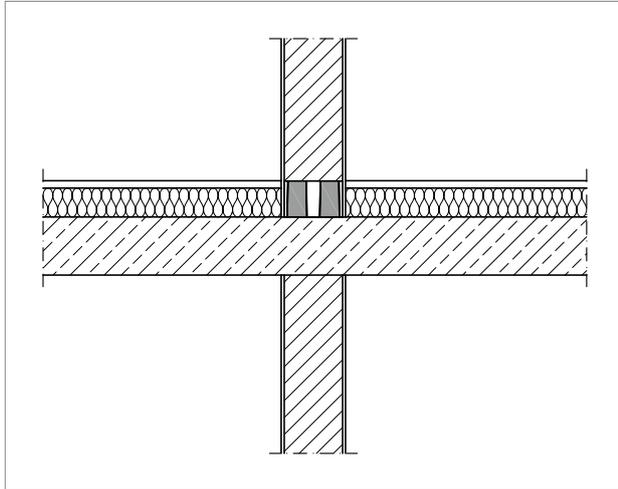
Fig. 54: Representation of a sectional drawing with detailed Schöck Sconnex® model
