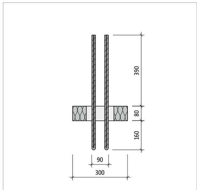
Fig. 90: Schöck Sconnex® type W-N-VH: Product section B-B
