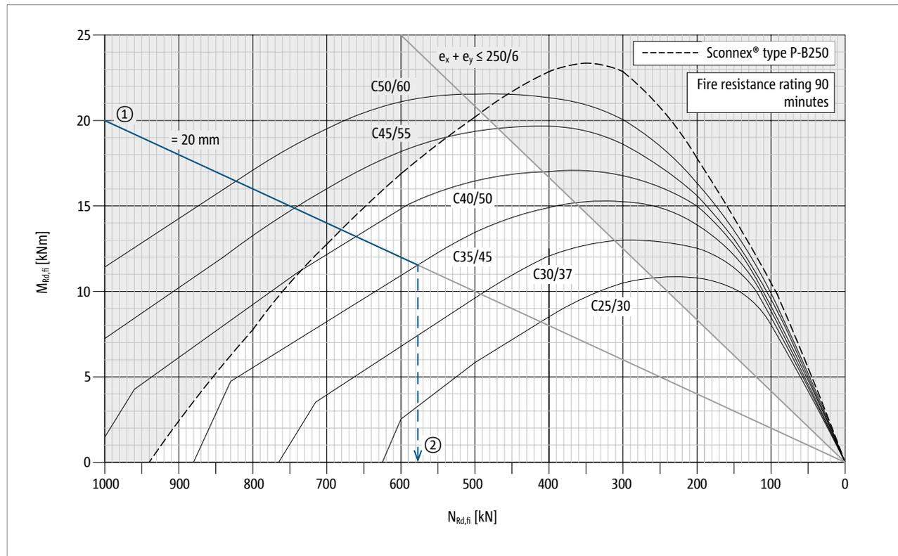
Fig. 182: Schöck Sconnex® type P-B250: Interaction diagram for the dimensioning for the case of fire, fire resistance class R 90
