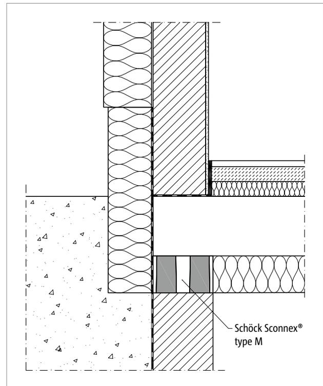
Fig. 188: Schöck Sconnex® type M: Installation condition below the basement floor
