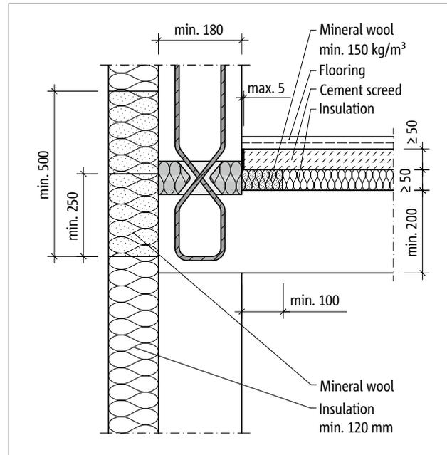
Fig. 97: Schöck Sconnex® type W: For combustible ETICS (exterior) with fire bar and edge strips made of mineral wool in the area of impact sound insulation
