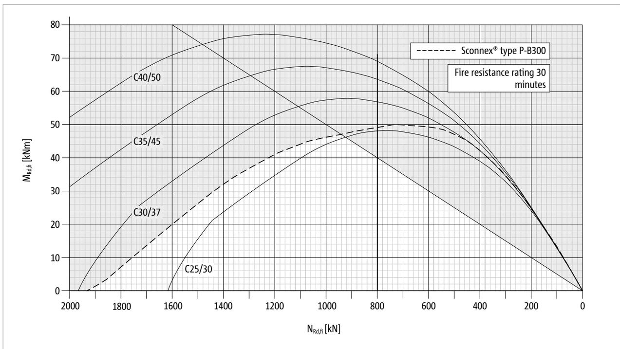
Fig. 134: Schöck Sconnex® type P-B300: Interaction diagram for the dimensioning for the case of fire, fire resistance class R 30
