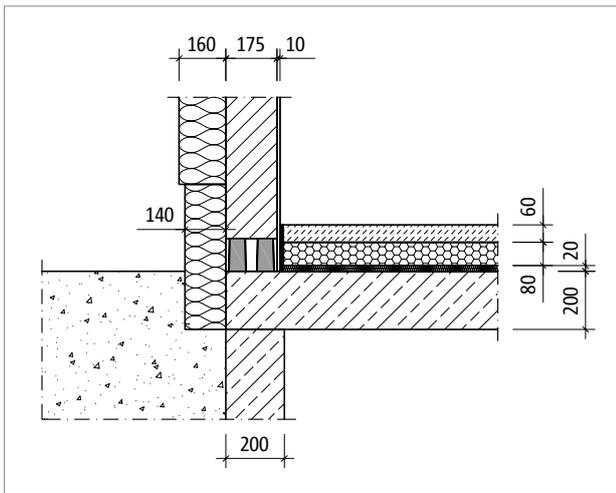
Fig. 52: Efficient thermal insulation using Schöck Sconnex® type M
