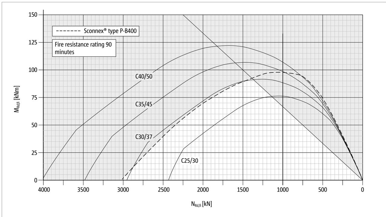
Fig. 138: Schöck Sconnex® type P-B400: Interaction diagram for the dimensioning for the case of fire, fire resistance class R 90
