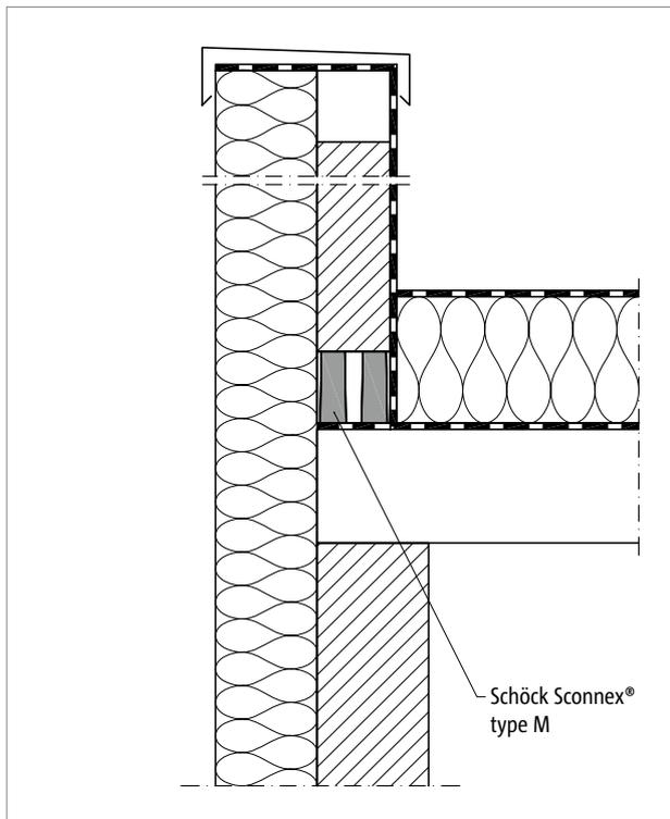
Fig. 187: Schöck Sconnex® type M: Installation condition in a parapet
