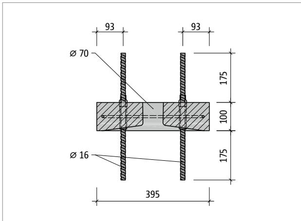
Fig. 161: Schöck Sconnex® type P-B400: Product section Part C
