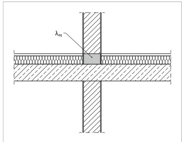
Fig. 39: Representation of a sectional drawing with simplified substitute insulating element
