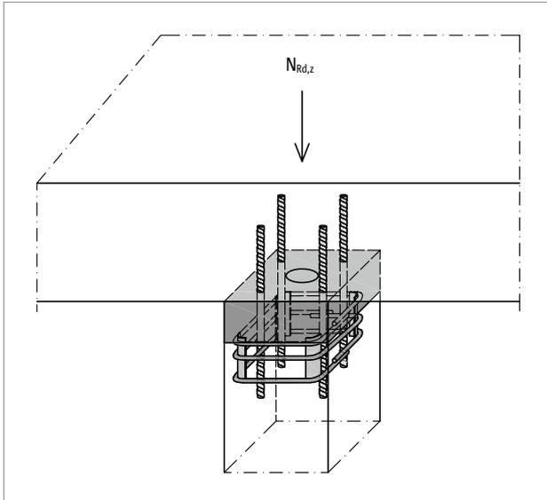
Fig. 181: Schöck Sconnex® type P: Sign convention for the design
