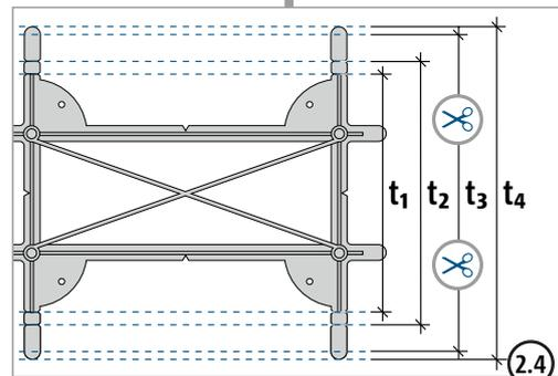
t<sub>1</sub> = 180 mm, t<sub>2</sub> = 200 mm, t<sub>3</sub> = 240 mm, t<sub>4</sub> = 250 mm
