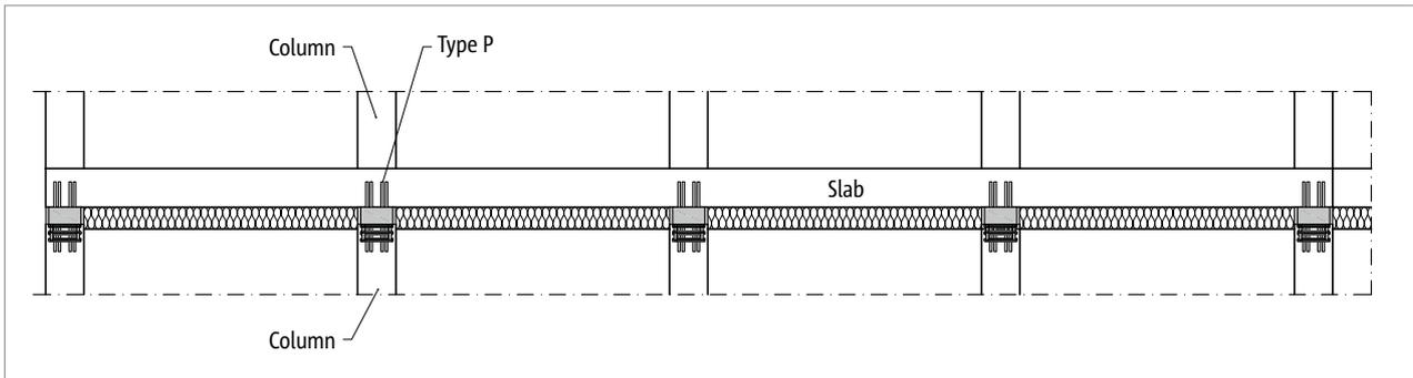
Fig. 117: Schöck Sconnex® type P: Column connection to the floor above
