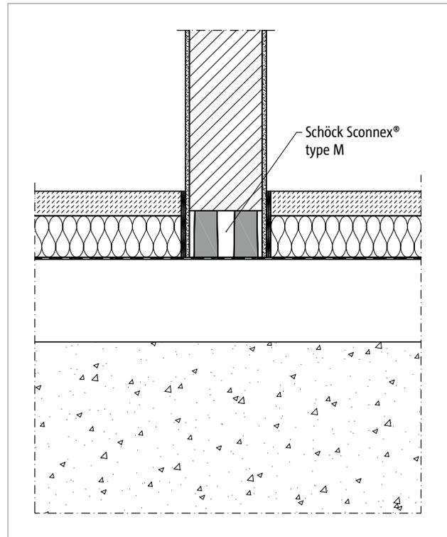
Fig. 190: Schöck Sconnex® type M: Installation condition with internal wall and foundation slab
