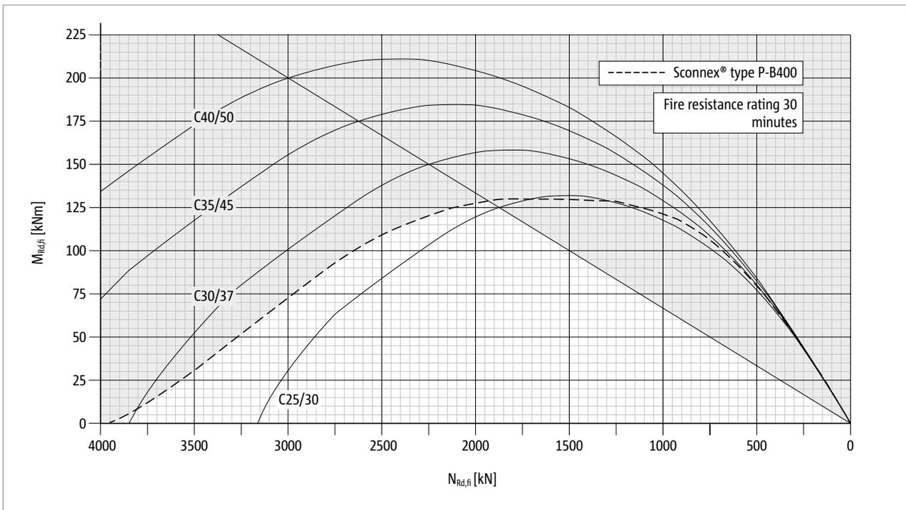
Fig. 140: Schöck Sconnex® type P-B400: Interaction diagram for the dimensioning for the case of fire, fire resistance class R 30
