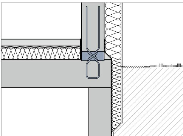
A reduction of the insulation thickness in the basement can take place via the offset between basement and ground floor wall. This reduces the costs and leads to a gain in useful area in the basement.
